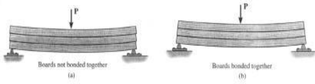
Figure 3.6 Action of shear stresses in unbonded and bonded boards
